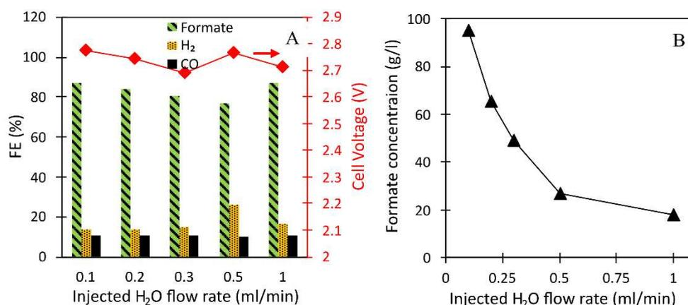
**Figure 4.** (A) Average FE towards formate and cell voltage of an interdigitated based zero-gap electrolyzer at  $100 \text{ mA/cm}^2$  and water injection flow rates varying between 0.1 and 1 ml/min at a  $CO_2$  flowrate of 200 ml/min for 1 h, 20 ml/min 2M KOH was fed to the anode side of the cell. (B) Effect of water injection flow rate on formate concentration.
