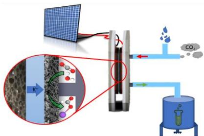
In this work, the effect of direct water injection on catholyte free zero-gap CO<sub>2</sub> electrolyzers is discussed. A novel method for the water injection is proposed and a theoretical description of the water balance inside the electrolyzer is provided. Furthermore, the influence of process conditions and long term stability is investigated. After optimization, formate concentrations up to 60 g/l at 100 mA/cm<sup>2</sup> and 2.7 V full cell potential were achieved.
