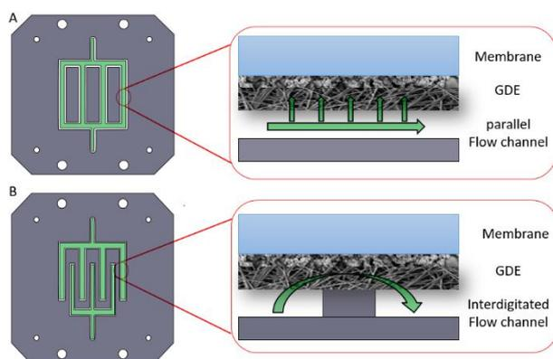
**Figure 2.** Schematic of the flow field patterns of the zero-gap electrolyzer: (A) parallel pattern where mass transfer is due to diffusion and (B) interdigitated pattern where mass transfer is a combination of diffusion and convection.
