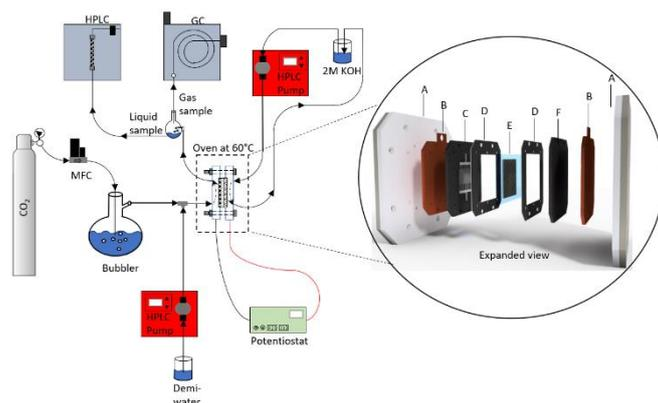
**Figure 1.** Experimental set-up of the zero-gap electrolyzer with direct water injection for optimized water management. Expanded view: (A) end-plates; (B) current collectors; (C) anode flow channel; (D) gaskets; (E) MEA; (F) cathode flow channel.
