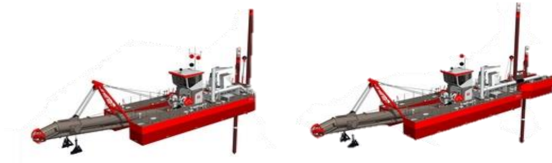
Figure 9: Dredger with(out) spud wagon
