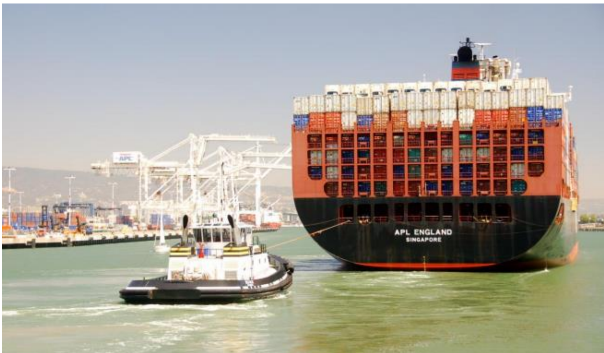
Figure 117: APL England with operating scrubber to the right of the funnel.
