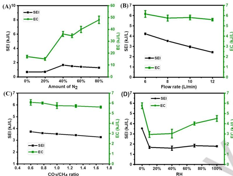
**Figure 5.** SEI and EC as a function of gas composition, gas flow rate and RH. (A) Total gas flow rate = 10 L/min,  $N_2$  fraction in  $CO_2$  varied from 0% to 80%. (B) The total gas flow rate varied from 6 to 12 L/min,  $CO_2/CH_4/N_2 = 1/1/8$ . (C) Total gas flow rate = 8 L/min,  $N_2 = 6.4$  L/min,  $CO_2/CH_4$  ratio varied between 0.6 and 1.67. (D) Total gas flow rate = 8 L/min,  $CO_2/CH_4/N_2 = 1/1/8$ ,  $H_2O$  amount varied between 0% and 100% RH.
