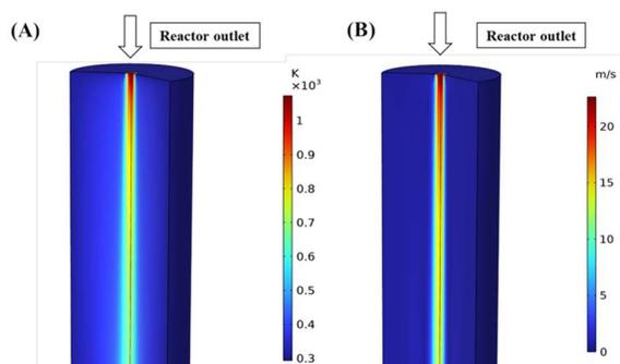
**Figure 8.** (A) Calculated gas temperature profile and (B) calculated flow velocity profile in the post-plasma reactor tube for a 1/1/8  $CO_2/CH_4/N_2$  mixture gas mixture and a flow rate of 8 L/min.
