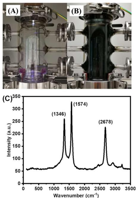
**Figure 4.** Photographs of post-plasma reactor tube and the Raman spectrum of the solid carbon product collected from the GAP DRM in the (B) case, at a total gas flow rate of 8 L/min,  $N_2 = 6.4$  L/min, for (A)  $CO_2/CH_4 = 1.67$ , (B)  $CO_2/CH_4 = 0.6$ , (C) Raman spectrum of carbon collected in the (B) case.
