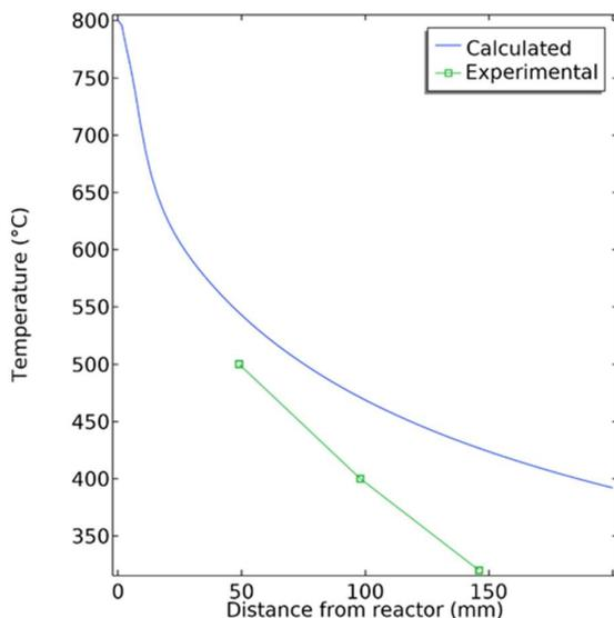
**Figure 9.** Comparison of temperature measured and modelled for the GAP reactor, as a function of distance from the reactor outlet, at a gas flow rate of 8 L/min and gas composition  $\text{CO}_2/\text{CH}_4/\text{N}_2 = 1/1/8$ .
