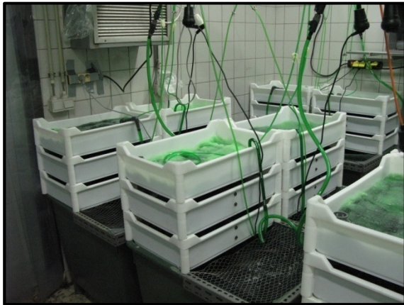
Fig. 9 Exposure aquaria with trickling filters at the University of Antwerp.
