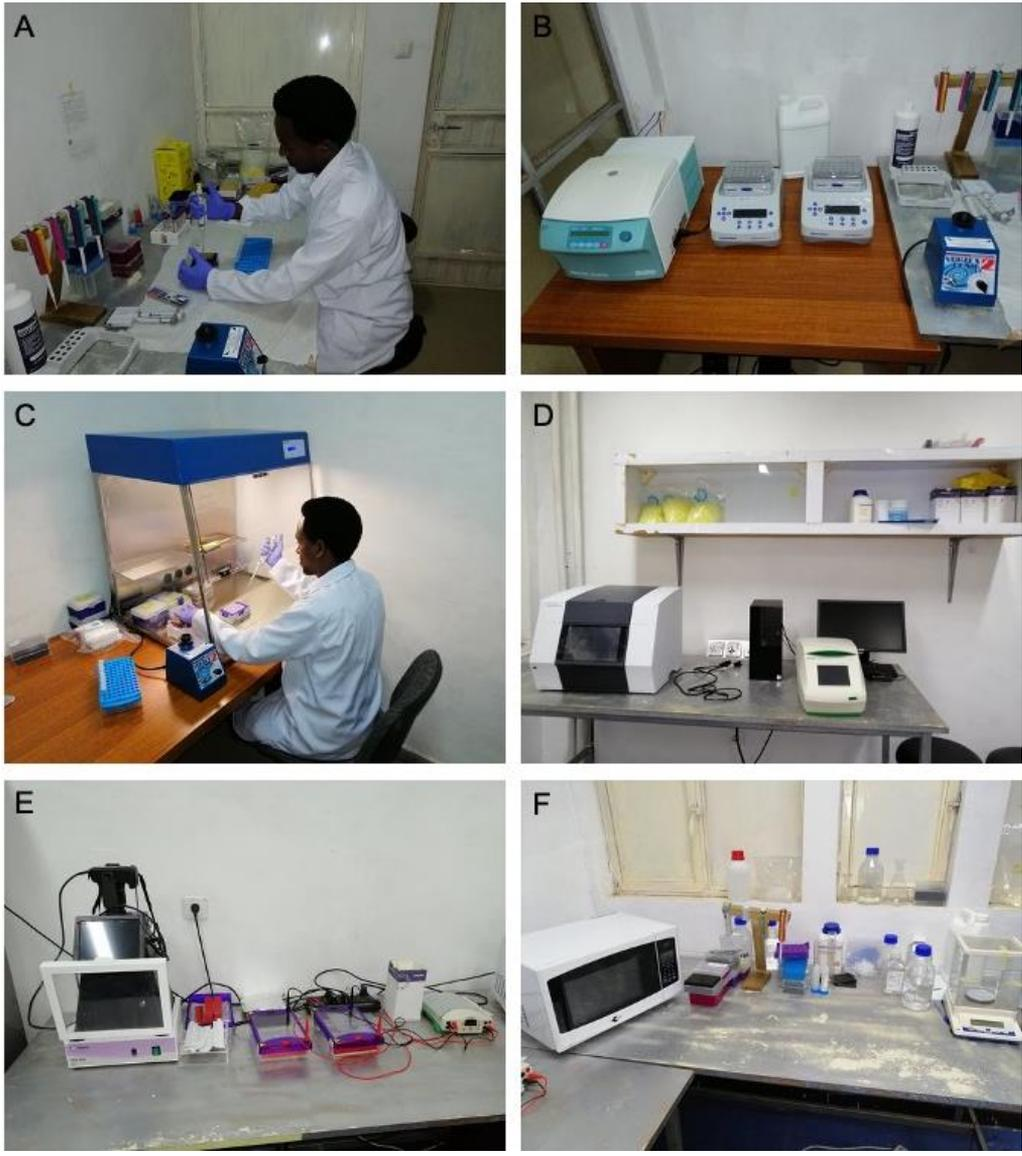
**Molecular laboratory at Arba Minch University.** Panel A and B present the DNA extraction room, panel C and D the pre-PCR room and panel E and F the post-PCR room. *Pictures by Nigatu Girma.*
