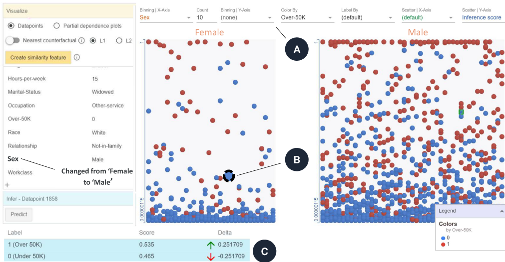
Figure 1.7: Interface of the "Datapoint Editor" component of the WhatIf tool. In (A) users can select which attributes of the data they want to visualize, using the x- and y-axis in a 2D graph, as well as the colours and labels for each datapoint. In this case "sex" is plotted on the x-axis, and prediction probabilities on the y-axis. This results into two graphs; one for women and one for men. Each point stands for one instance, and their colour denotes their ground truth label (high income - red, low income - blue), while their point in the y-axis denotes their obtained prediction probability (points on the x-axis are randomly spread to increase readability). Here we see, that generally fewer women are represented in the dataset, and it appears that women are more likely to obtain low prediction probabilities. In the graph, users can also select individual data points to either run a counterfactual or a what-if analysis on. (B) In this case, an auditor has selected a female datapoint, to observe how her prediction probability for a high income would be different if her sex was "male" instead. In (C) we see that the change in sex increases the prediction probability for a high income by \sim 0.25 , indicating a potential case of individual discrimination
