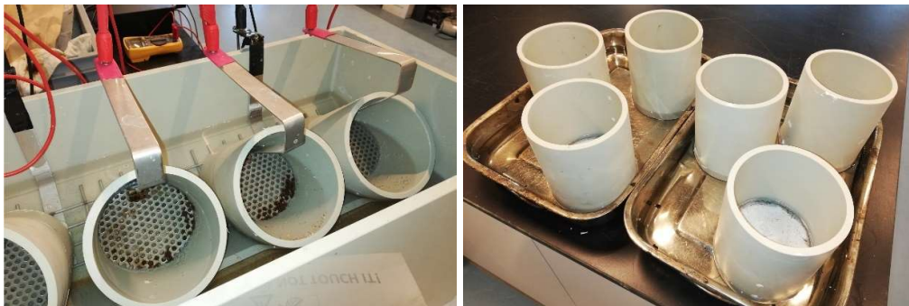
Fig. 3. The test setup for chloride migration.
