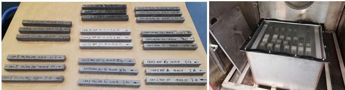
Fig. 4. The ASR samples (a) and curing setup (b).
