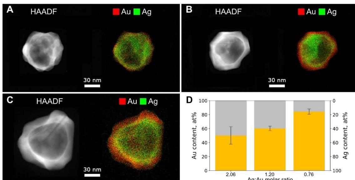
**Figure 2.** (A-C) Representative HAADF-STEM images and EDX maps of nanoparticles obtained for different Ag:Au molar ratios: 2.06 (A), 1.2 (B) and 0.76 (C). (D) Relative content of Au (yellow) and Ag (grey) in nanoparticles of samples at different Ag:Au molar ratios, as labeled. Error bars correspond to the standard deviation between measurements for 5 different nanoparticles.
