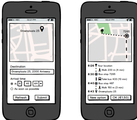
Figure 1: Mock-up of a mobile interface to a fully on-demand public bus system
