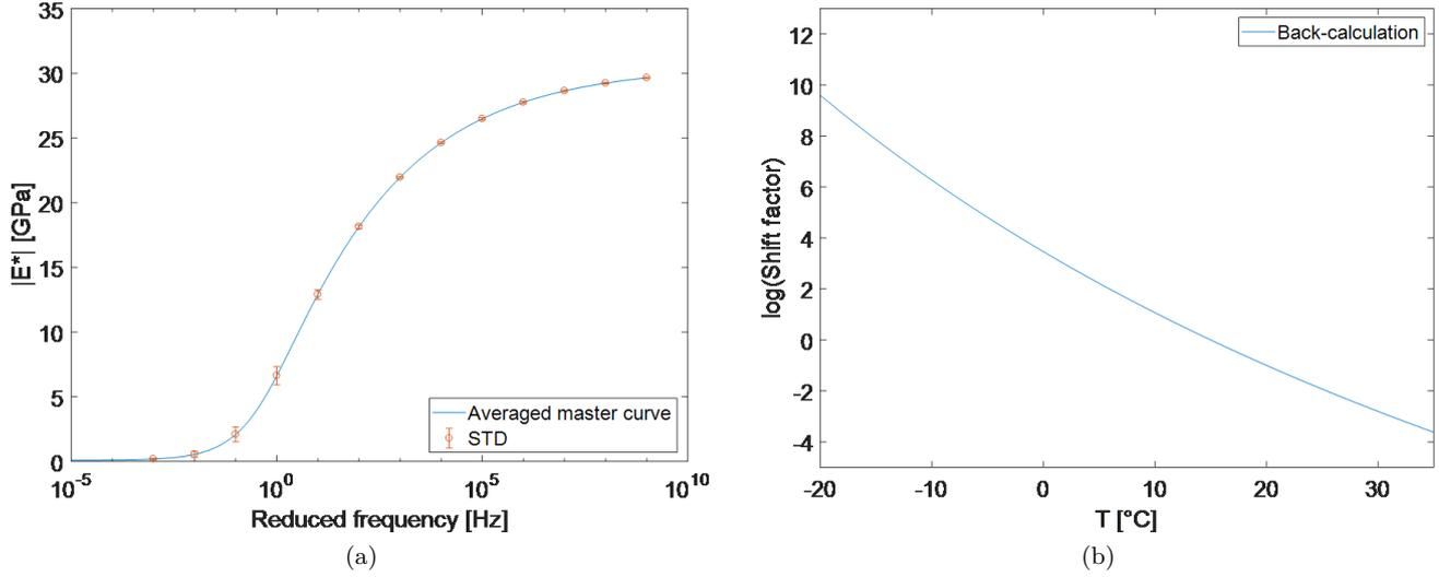
Fig. 5: (a) Averaged master curve of the specimens  $B1 - B3$ , at the reference temperature of  $15\text{ }^\circ\text{C}$  computed by the back-calculation technique, (b) the shift factor according to the WLF approach.
