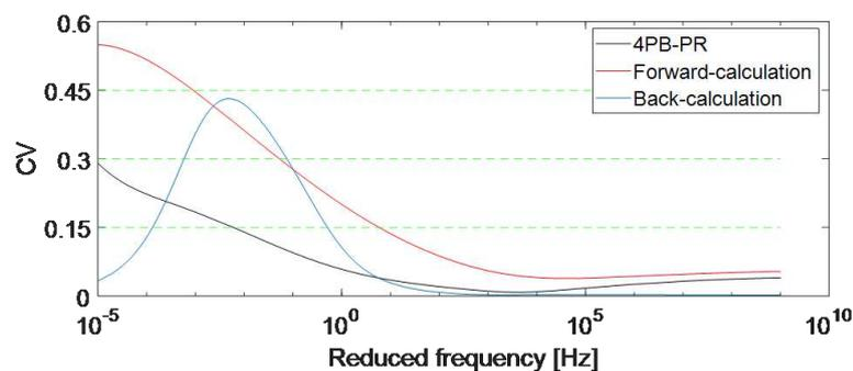
Fig. 8: Coefficient of variance computed for three different methods. All methods have high repeatability at frequencies higher than 10 Hz.
