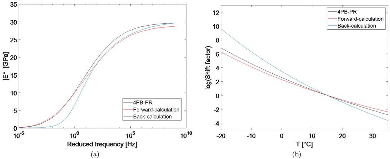
Fig. 6: (a) Comparison of the averaged master curves using three different methods at the reference temperature of  $15\text{ }^\circ\text{C}$ . (b) Comparison between the shifting factors derived using the three methods.
