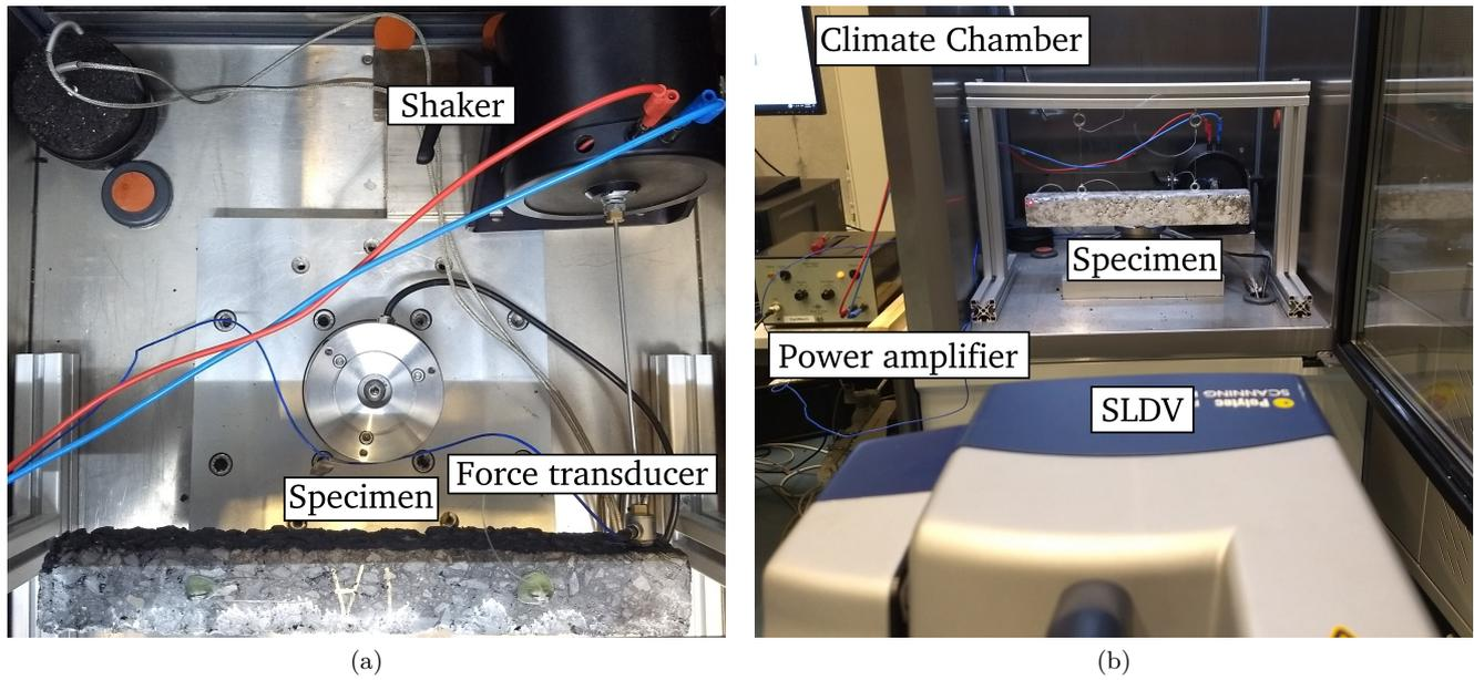
Fig. 3: Experimental setup: (a) Top view inside the climate chamber. (b) Overall view from the back of the SLDV.
