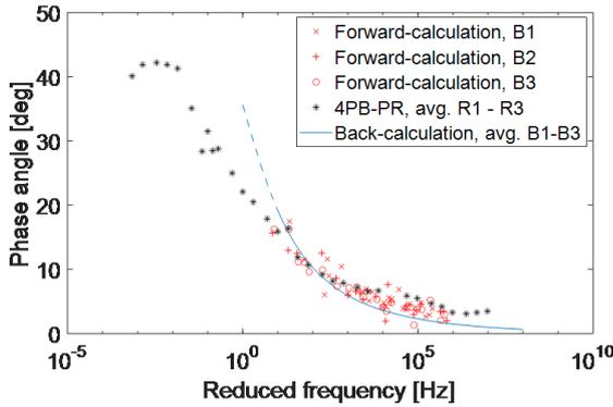
Fig. 7: Comparison of the phase angles derived from three methods at reference temperature of 15 °C. The result of the forward-calculation on three beams are presented separately since the natural frequencies of the beams are not the same, and therefore, it is not possible to take an average of the phase angles at certain frequencies.
