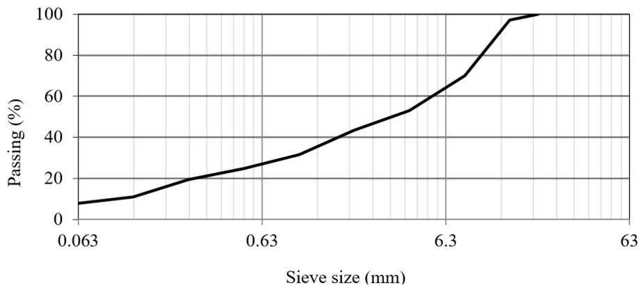
Fig. 2: Grading curve of the designed mixture.
