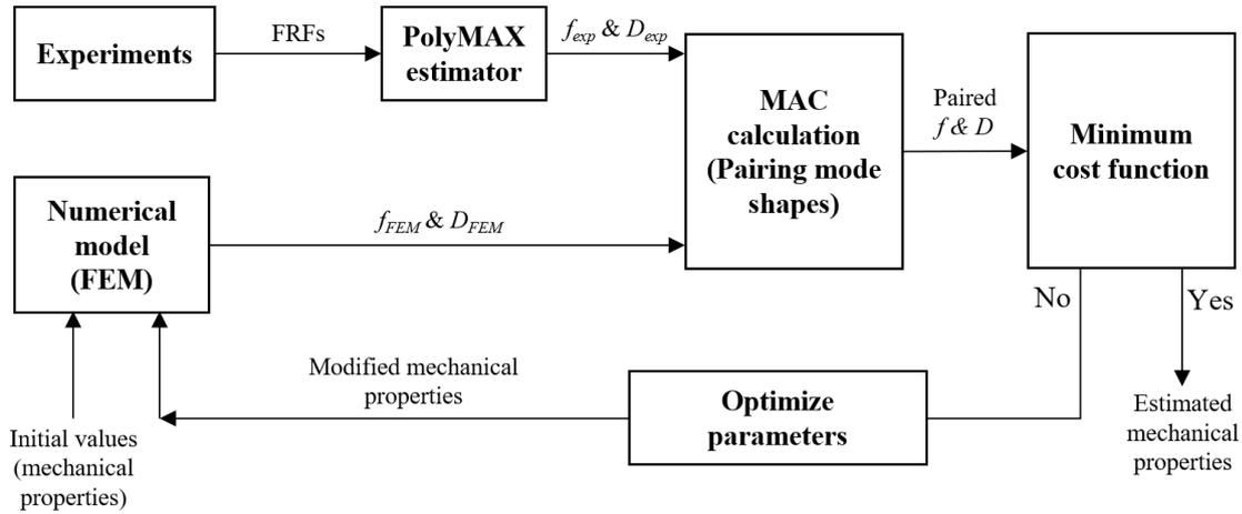
Fig. 4: Overview of the back-calculation methodology used in this research to find the desired properties of the pavement mixtures ( $f$  is the vector of natural frequencies, computed from  $\omega_k$ , and  $D$  is the vector of percentage of damping ratios, calculated from  $\xi_k$ ).
