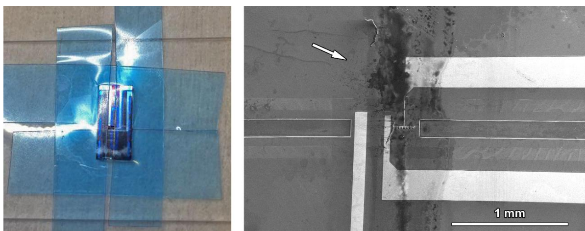
Figure 94. Illustration of the double-sided tape method we have tried. The left image is a photo of the tape used to cover the chip. The right image is an SEM image of how the chip looks after the deposition with the double-sided tape method.
