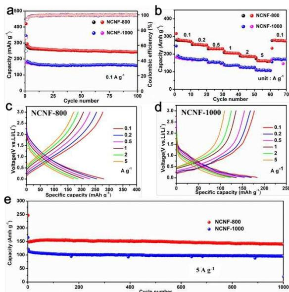
**Figure 3.** Electrochemical properties of the NCNF-800 and NCNF-1000. (a) Cycling performance of NCNF-800 and NCNF-1000 samples tested at a current density of 100 mA g<sup>-1</sup>. (b) Rate performance of NCNF-800 and NCNF-1000 at various current densities from 0.1 to 5 A g<sup>-1</sup>. (c, d) The corresponding charge and discharge voltage profiles of NCNF-800 and NCNF-1000 at different current densities. (e) Cycling performance of NCNF-800 and NCNF-1000.
