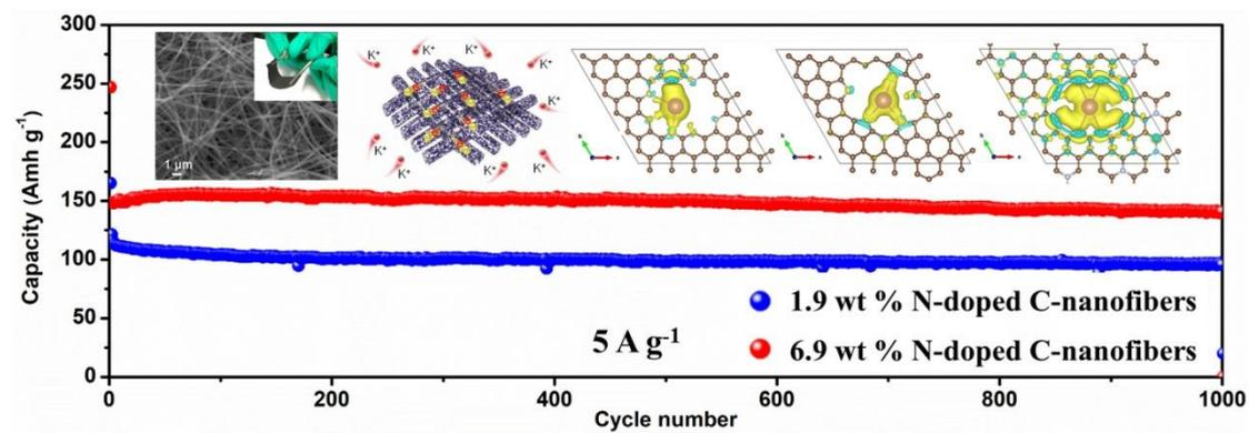
The origin of the extra capacity of freestanding and porous N-doped carbon nanofibers was clearly revealed by systematic experimental analysis and theoretical calculations.
