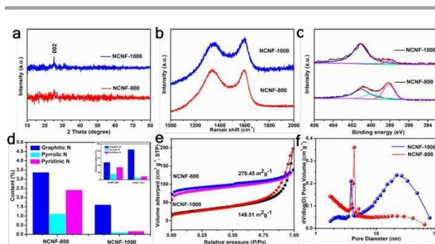
Figure 2. Structure characterization of porous NCNF-800 and NCNF-1000 samples. (a) XRD patterns. (b) Raman spectra. (c) High-resolution N 1s XPS spectra. (d) The corresponding contents of graphitic N, pyrrolic N and pyridinic N from (c). (e, f) BET and BJH curves.
