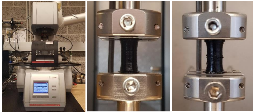
Figure 8: DSR MCR 102 (left), sample mounted in the SCF holder (middle) and a damaged sample after test completion (right).
