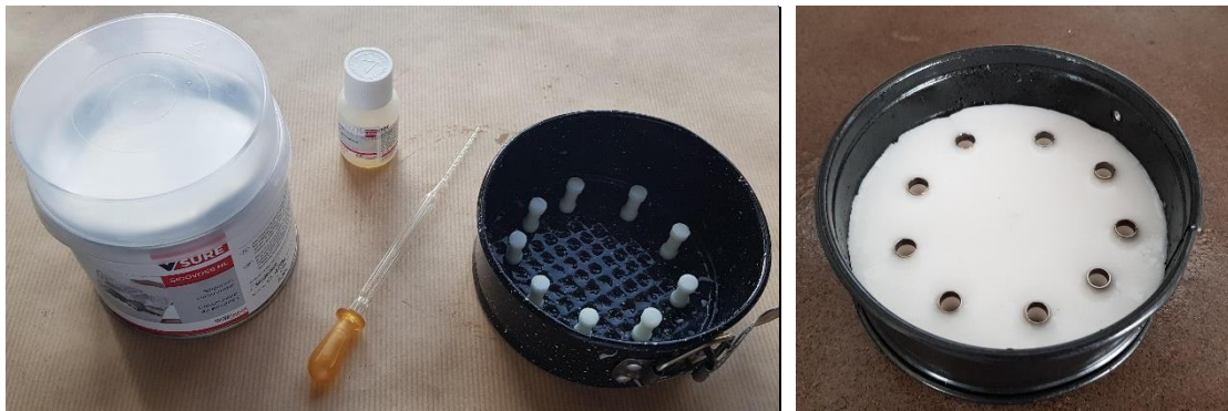
Figure 6: Preparation of casting mould: two-component casting silicone together with a spring-form and nine 3D-printed samples(left); ready-to-use casting silicone mould with steel rings (right).
