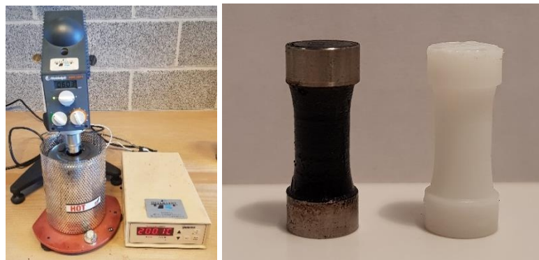
Figure 6: Preparation of casting mould: two-component casting silicone together with a spring-form and nine 3D-printed samples(left); ready-to-use casting silicone mould with steel rings (right).
