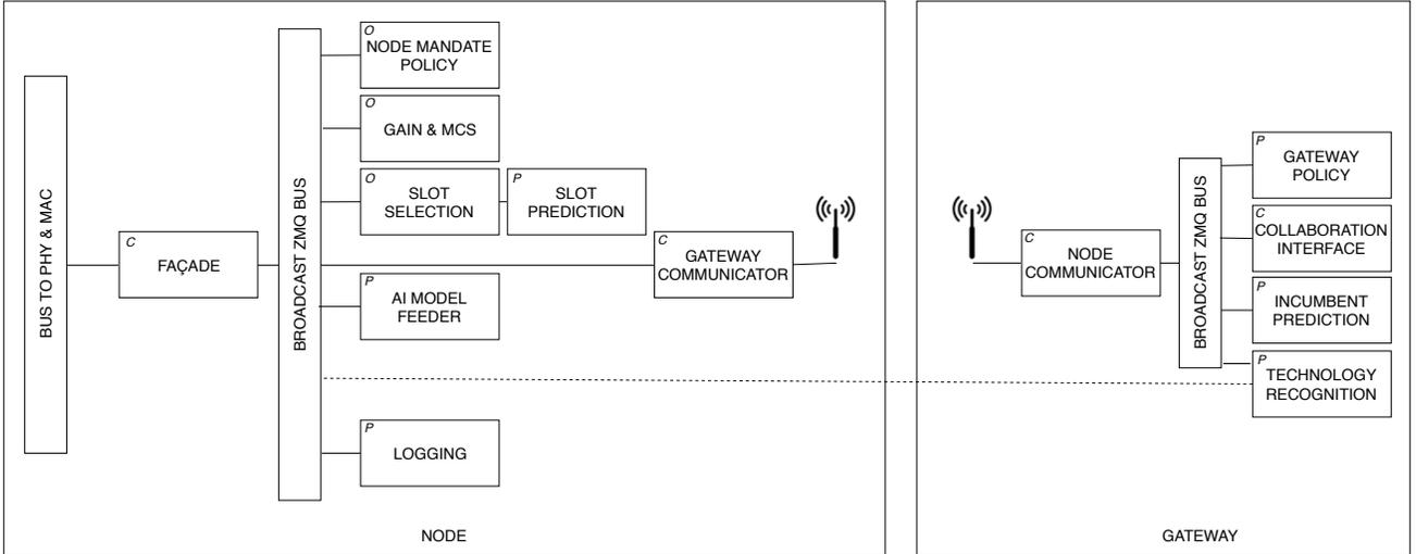
Fig. 4: Architecture of the decision engine of the SCATTER radio system, based on communication modules (annotated with C), optimization modules (annotated with O), and processing modules (annotated with P). The antenna represents a UDP socket that injects data into the own radio stack via the network interface.
