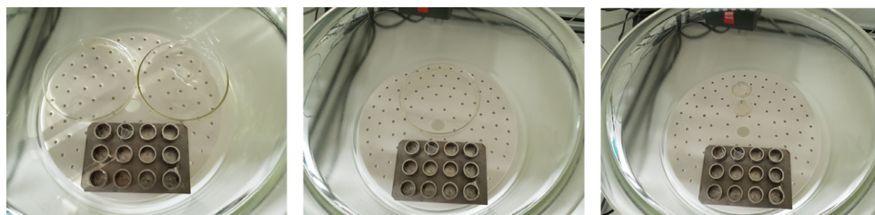
Fig. 1. Passive exposure of A549 cells using 2 Petri dishes filled with 6 ml gasoline each in a humidified desiccator in a climatic chamber at 37 °C.
