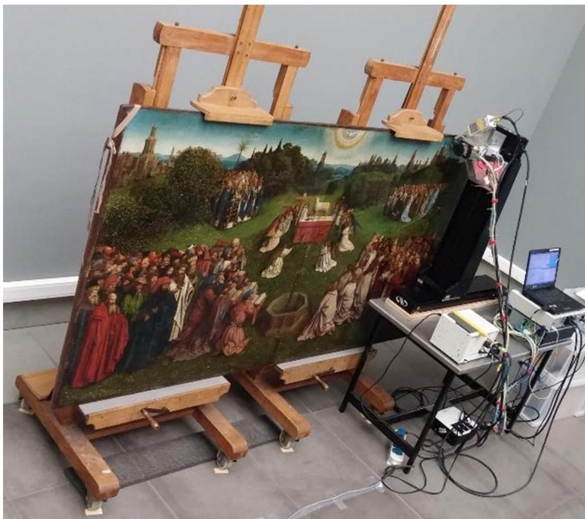
*Figure S2: Experimental setup. The MA-XRF instrument during experiments on the central panel (Adoration of the Lamb). "Geert Van der Snickt at University of Antwerp".*
