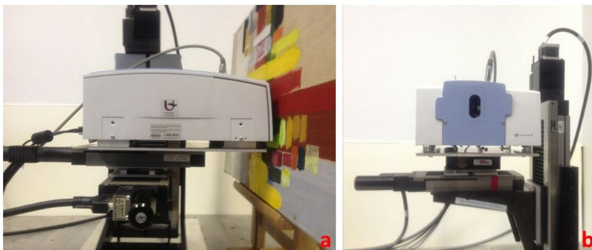
Figure 1: Photographs of the MA-FTIR scanning setup: (a) side- and (b) front view.
