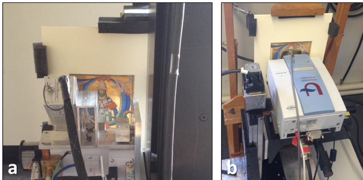
Figure 2: (a) MA-XRF scanning of MS 5–1979; (b) MA-rFTIR scanning of MS 5–1979. In both cases, the measuring head is positioned on a motorized two-dimensional stage while the manuscript fragment is securely mounted on an easel and remains stationary.
