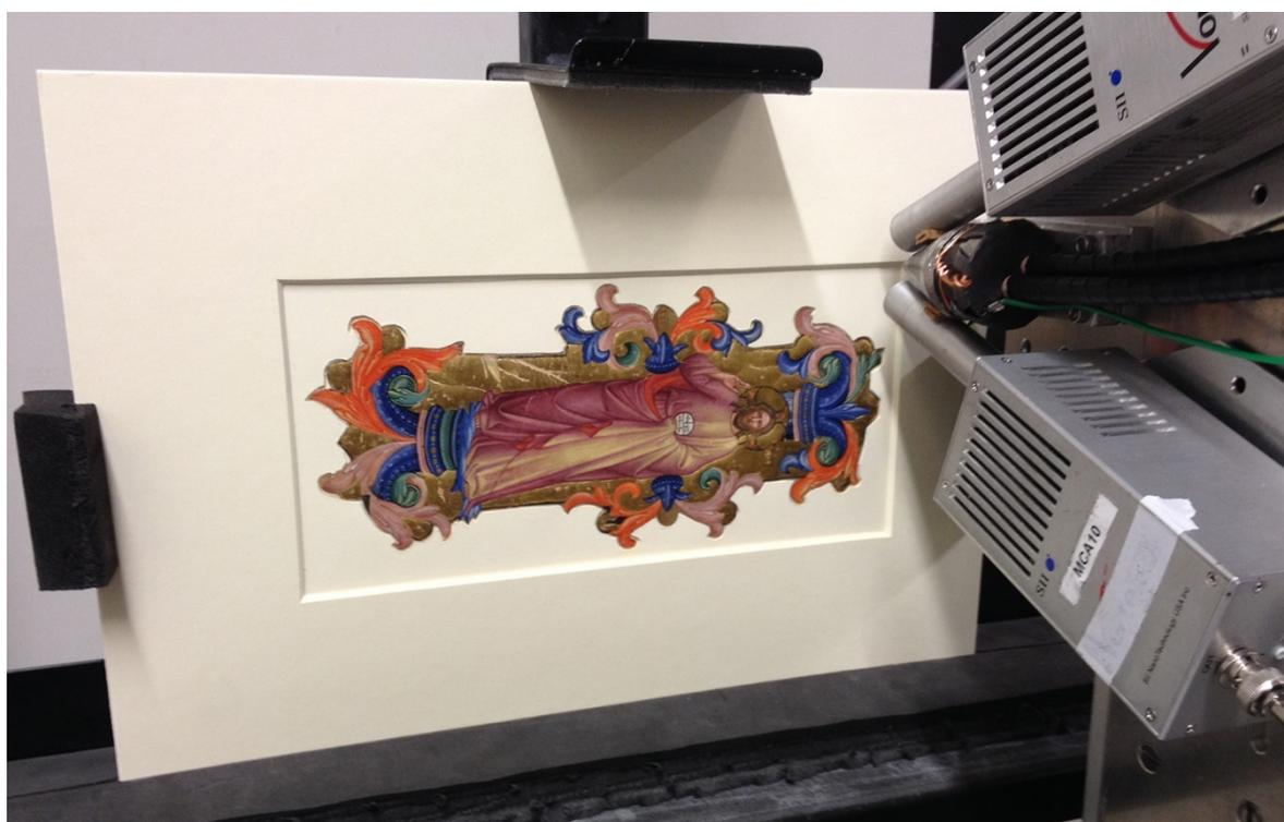
*Figure 2: Detail of the MA-XRF scanning head in front of a mounted manuscript fragment (Fitzwilliam Museum, Marlay Cutting It 13ii).*
