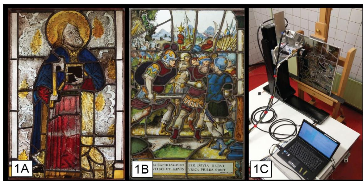
Figure 1: – The studied glass panels from the collection J. M. A. Caen, Schoten, Belgium. **1A**: St Matthew, England, early 15<sup>th</sup> century. **1B**: The Arrest of King Zedekiah, Brabant (Leuven), by Jan de Caumont (c. 1580-1659). **1C**: the MA-XRF instrument of the University of Antwerp during scanning of The Arrest of King Zedekiah.
