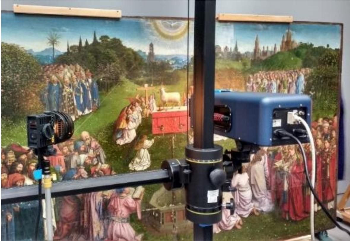
*Figure S3: Experimental setup. Near-infrared reflectance imaging spectroscopy (~980-1680 nm). "Kathryn Dooley at National Gallery of Art".*
