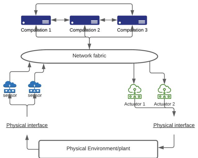
FIGURE 1. Example structure of a CPS (adapted from [12]).
