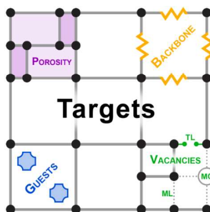
Figure 3. MOF's functionality targets: porosity, backbone, guests, and framework vacancies. Different types of vacancies can be distinguished (ML= missing linker; MC= missing cluster; TL= 'truncated linker').
