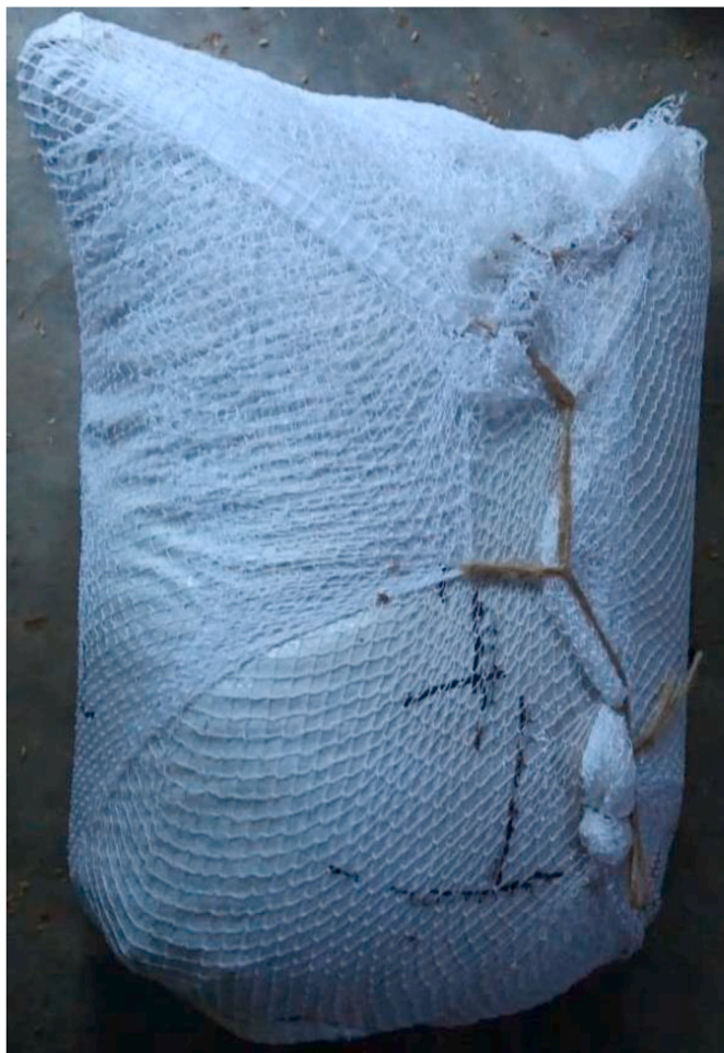
Fig. 2. Polyethylene bag used for the assessment of post-harvest rodent damage to stored rice. Treatment bags were enclosed in fishnet with mesh size of 1.5 \times 1.5 cm double layer to protect rice grain from rodent damage. Control bags were without fishnet (not shown).
