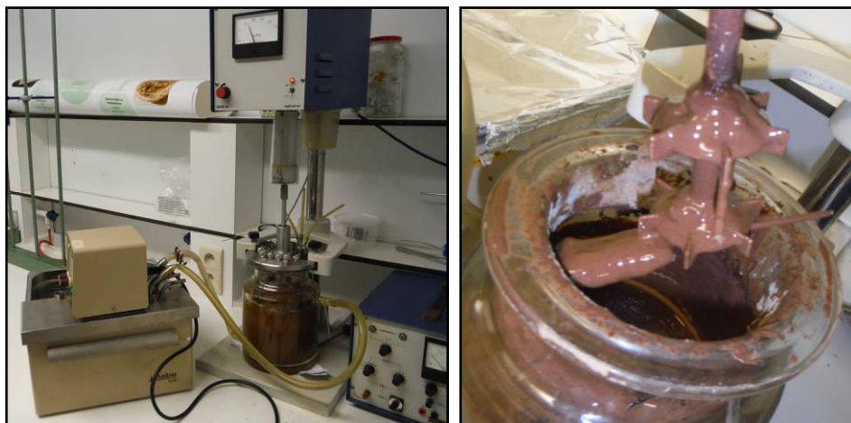
Figure 5-9: Setup used for viscous medium fermentations (left) and the rotor with the attached magnet (right).
