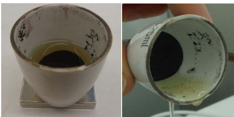
Figure 4-1: (left) m-CLEAs sedimentation with a magnet. (right) Decantation of the liquid from the catalyst.
