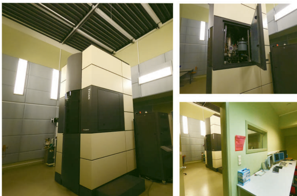
FIGURE 1.5: Left, EMAT double corrected Thermo Fisher Scientific TITAN 3 microscope. Upper right, access to the side-entry stage. Bottom right, control room.
