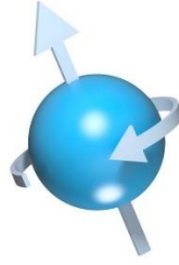
Figure 3.10: Spinning electron with magnetic moment through its center.
