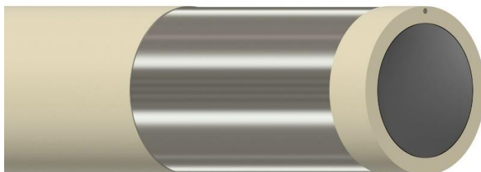
Figure 11.1: Optimized GC electrode for standard EPR tube.
