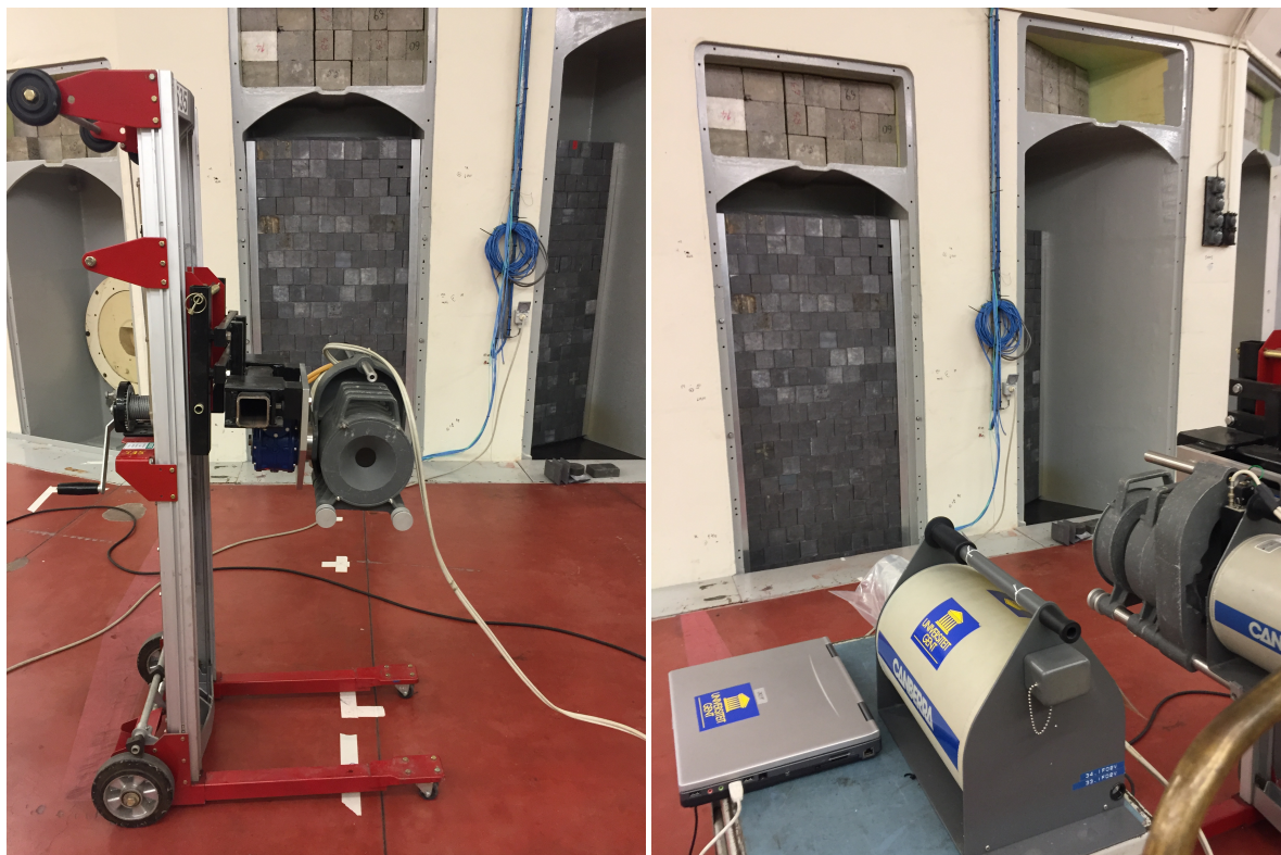
Figure 11.2.1: Germanium detectors, provided by SCK-CEN (left) and provided by Ghent University (Right)
