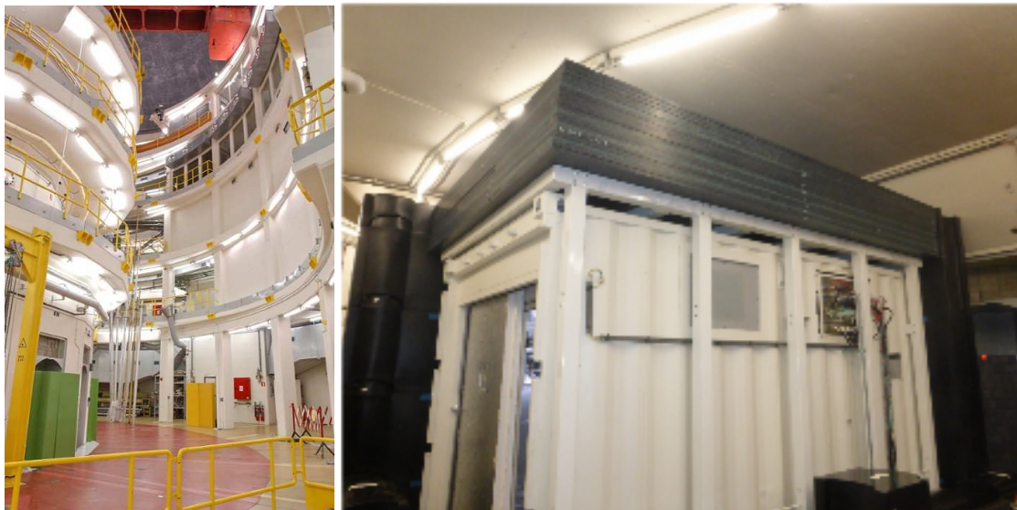
Figure 5.0.4: Left: Hall of BR2 reactor building where the SoLid detector is located. Right: The detector and its passive shielding.
