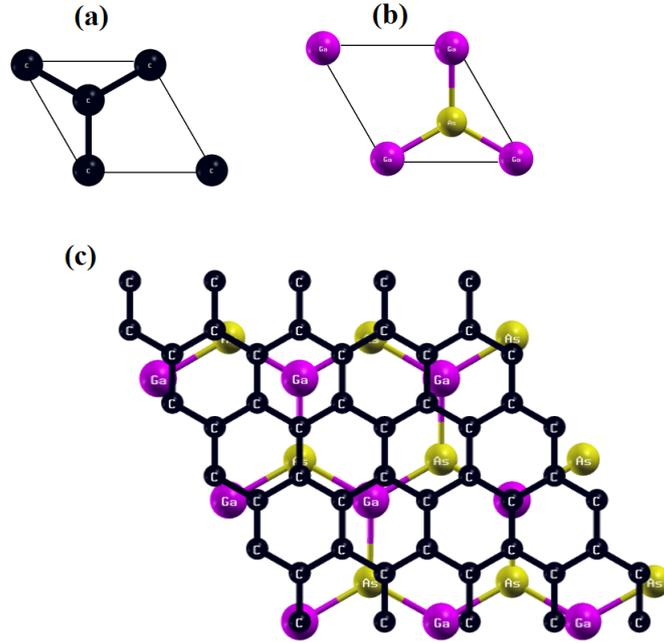
Figure 4-2: Honeycomb unit cells for (a) Graphene, (b) 2D-GaAs monolayers, and (c) 551-Graphene/331 GaAs bilayer crystal heterostructure.
