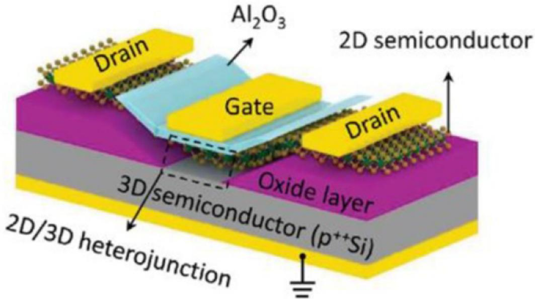
Figure 1-13: Schematic diagram of a tunneling field-effect transistor based on a vertical heterostructure of 2D MoS<sub>2</sub>, and 3D Si and Group III-V semiconductors [11].
