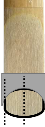
Figure 3: Top view on a reed with the artificial lip in place. The black line indicates the circumference of the zone in which 3D vibration data are measured. The dotted lines indicate the locations of cross sections along which reed motion will be shown (Section III.C). The artificial lip is indicated with gray. (color online)
