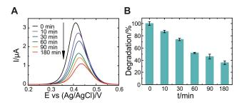
**Fig. 4.** Baseline corrected square wave voltammograms of **A)** 100 μM PHOH in pH 12 BR after anodic pretreatment at 0.9 V over time (from 0 to 3 hours). Corresponding degradation plot of **B)** PHOH over time (N=3).
