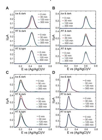
**Fig. 3.** Baseline corrected square wave voltammograms of 10  $\mu$ M phenols in pH 12 BR, **A)** PHOH, **B)** PCP, **C)** OP and **D)** BPA. Stability of different stocks over the time (from 0 to 5 hours) stored in ice and dark; at room temperature and dark; and at room temperature and daylight.
