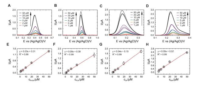
**Fig. 5.** Baseline corrected square wave voltammograms for **A)** PHOH, **B)** PCP, **C)** OP and **D)** BPA in pH 12 Britton Robinson buffer in a concentration range from 1 to 50 μM using Italsens SPE (N=3). Corresponding calibration curves of all phenols **E)** PHOH, **F)** PCP, **G)** OP and **H)** BPA showing the average of the peak current upon increasing concentrations of each phenol (N=3).
