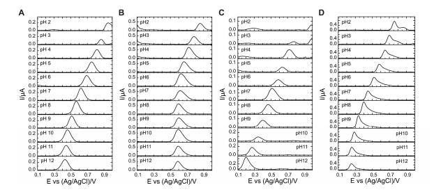
**Fig. 2.** Baseline corrected square wave voltammograms of 10 μM concentration of phenols: **A)** PHOH, **B)** PCP, **C)** OP and **D)** BPA; obtained during pH screening in Britton Robinson buffer (20mM and 0.1 mM KCl, in the pH range 2 to 12) on Italsens SPE.
