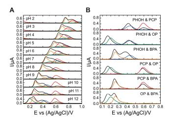
**Fig. 6**. Baseline corrected square wave voltammograms obtained after **A)** pH screening (pH 2 to 12) in Britton Robinson buffer of the complex mixture (black line) using 10 μM concentration of each phenol (1:1:1:1 ratio) and **B)** binary mixture of phenols (black line) of 10 μM concentration of each phenol (1:1 ratio) in pH 12. Single phenol solutions of PHOH (blue line), PCP (red line), OP (green line) and BPA (orange line) were also provided.
