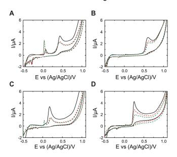
**Fig. 1.** Cyclic voltammograms of **A)** PHOH, **B)** PCP, **C)** OP and **D)** BPA using 100 μM concentration in pH 12 Britton Robinson buffer at Italsens SPE. First scan (black line), second scan (red dotted line) and third scan (green dotted line). Three consecutive scans were performed within the same phenol droplet.
